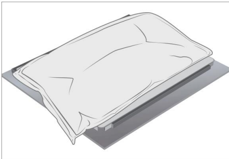
Place 9 kg steel shot bag onto device
